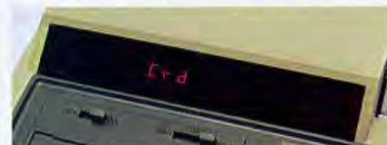
*If the second side of a card is required, the calculator displays "Crd."*
