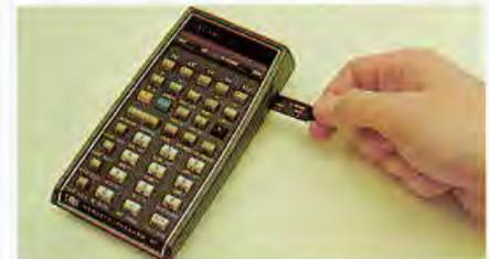
Pre-recorded program cards are easily entered into the HP-67 in the slot on the right side.
