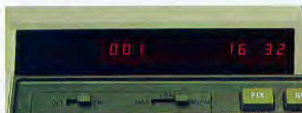
This operation occupies the first step of program memory as indicated by the step number 001. The keycode 16 identifies the sixth key in the first row of the left block of keys (f). The keycode 32 identifies the second key in the third row of the left block of keys (LOG). Keys from the right side of the HP-97 keyboard are preceded by a minus sign.
