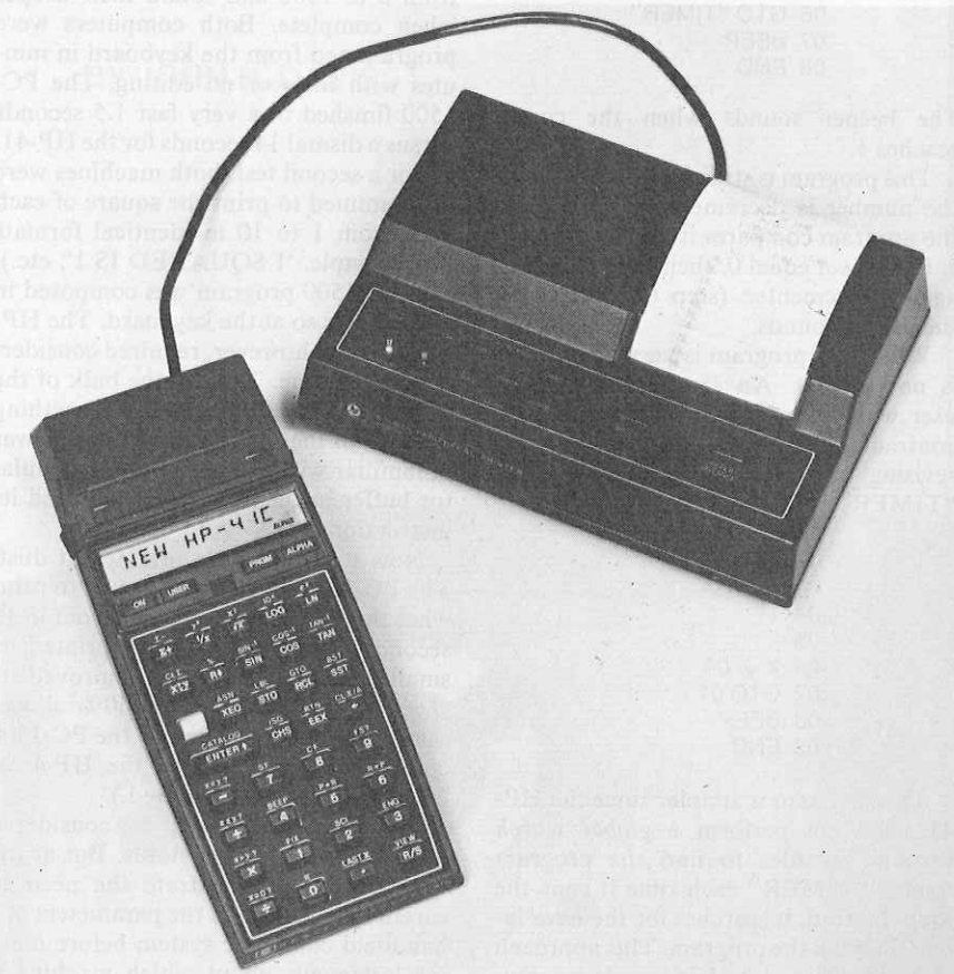
The HP-41C shown here is generating the function sine x. The output, with the curve, is shown on the printer.
