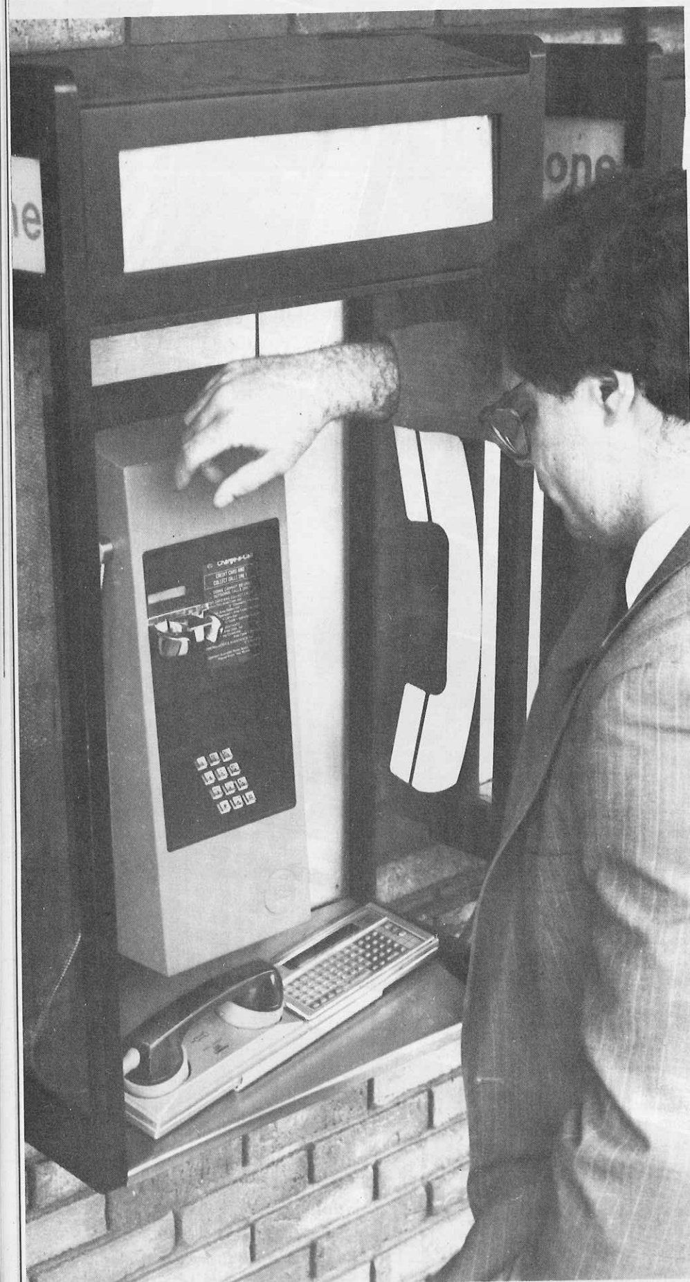
The Quasar HHC telephone modem can be used in the field to access a network or home-based computer.
