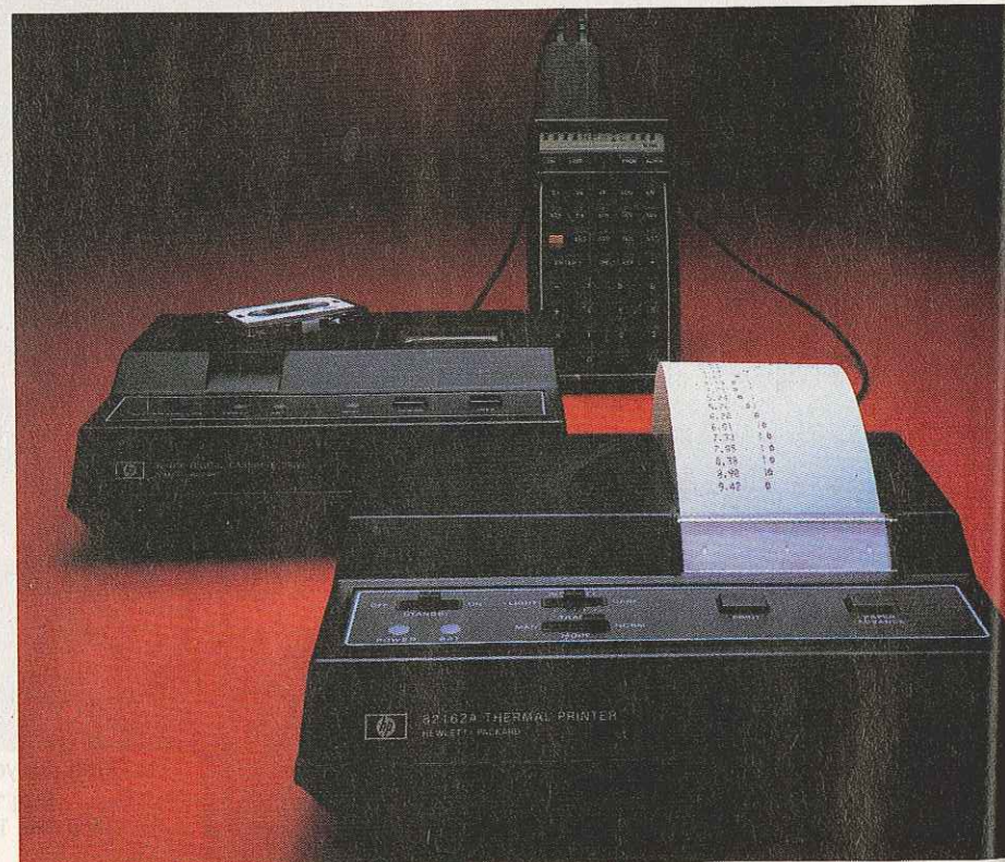
The HP-IL Interface Loop enables the HP-41 to be used with a number of peripherals. Shown are Cassette Drive and Printer.
