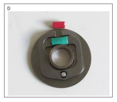
Picture C shows the assembly. In picture D it is mounted in the mechanism. Now there is no play while still there is flexibility in the mount.
