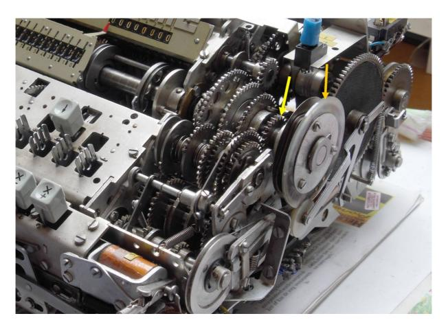
The plastic dish (see orange arrow) on the above photo is attached to a toothed wheel (not visible here) which connects the gearbox shaft in the back with either the Reg-I rotor or the mechanism which in lateral direction transports Reg-I back to its initial position after addition or subtraction.
